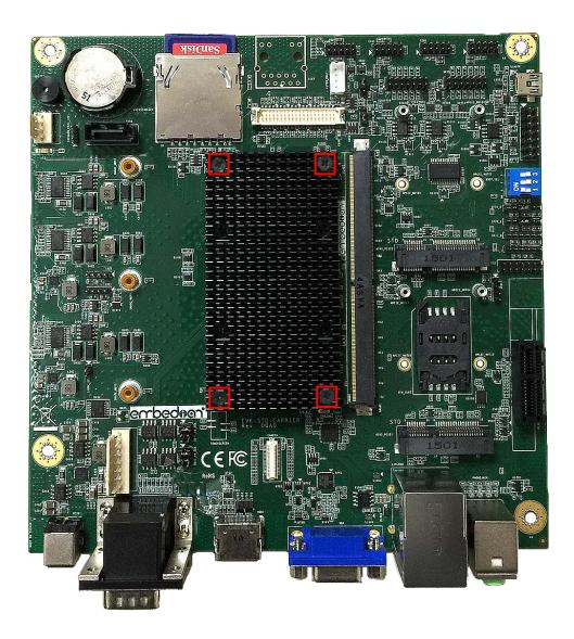
7. For application which results in the prolonged overheating of the processor, either due to environmental condition (like higher ambient temperature) or due to very high computational power; the DC fan can be mounted on the top of the VTT-HS-8J064 SMARC Module Heatsink using M3 screws (4 units). The mounting holes for DC fan are compatible to FAD1-04010BBLW11 from Qualtek Electronics and is available from Digikey (P/N: Q608-ND).
