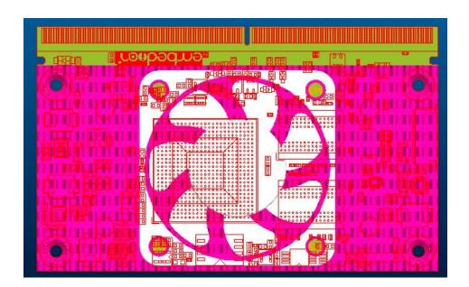
For the majority of the end applications, an additional heatsink fan will not be required.
