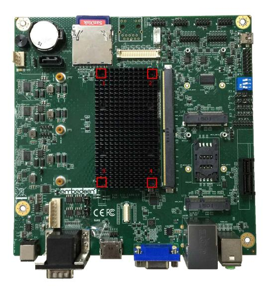
5. Use 4 units of M2.5 12mm sized screws to affix the heatsink together with the system.
